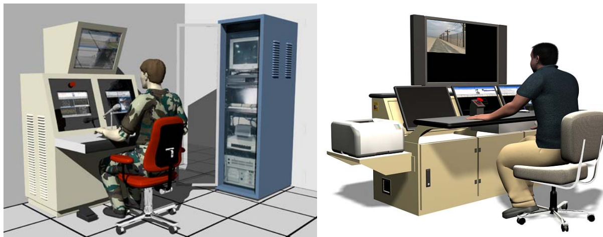
Figure 4. Modernized and Simplified Control Station Design (Shown on Right) Combines Console and Equipment Rack in a Single Unit.
